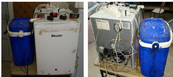
Fig.2: Domestic Refrigerator with Water Heater Tank photograph.
